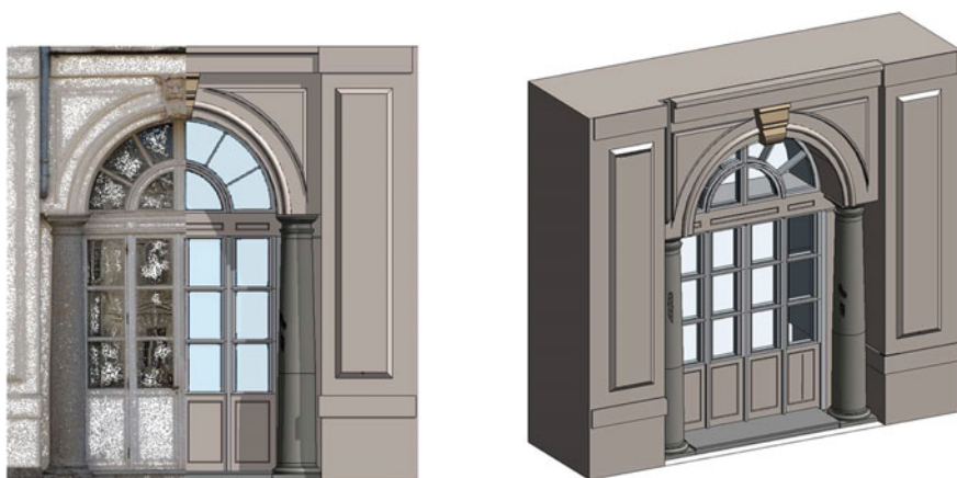
Fig. 3 Point cloud comparison with a historical building object model (H-BOM)
