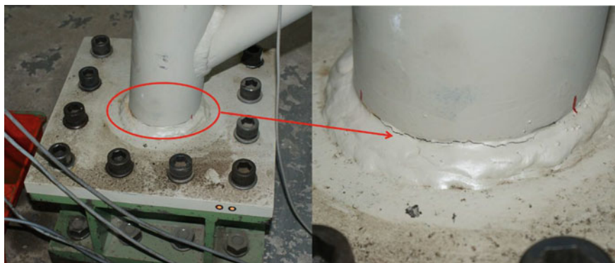
Fig. 4 First fatigue crack at one jacket foot
